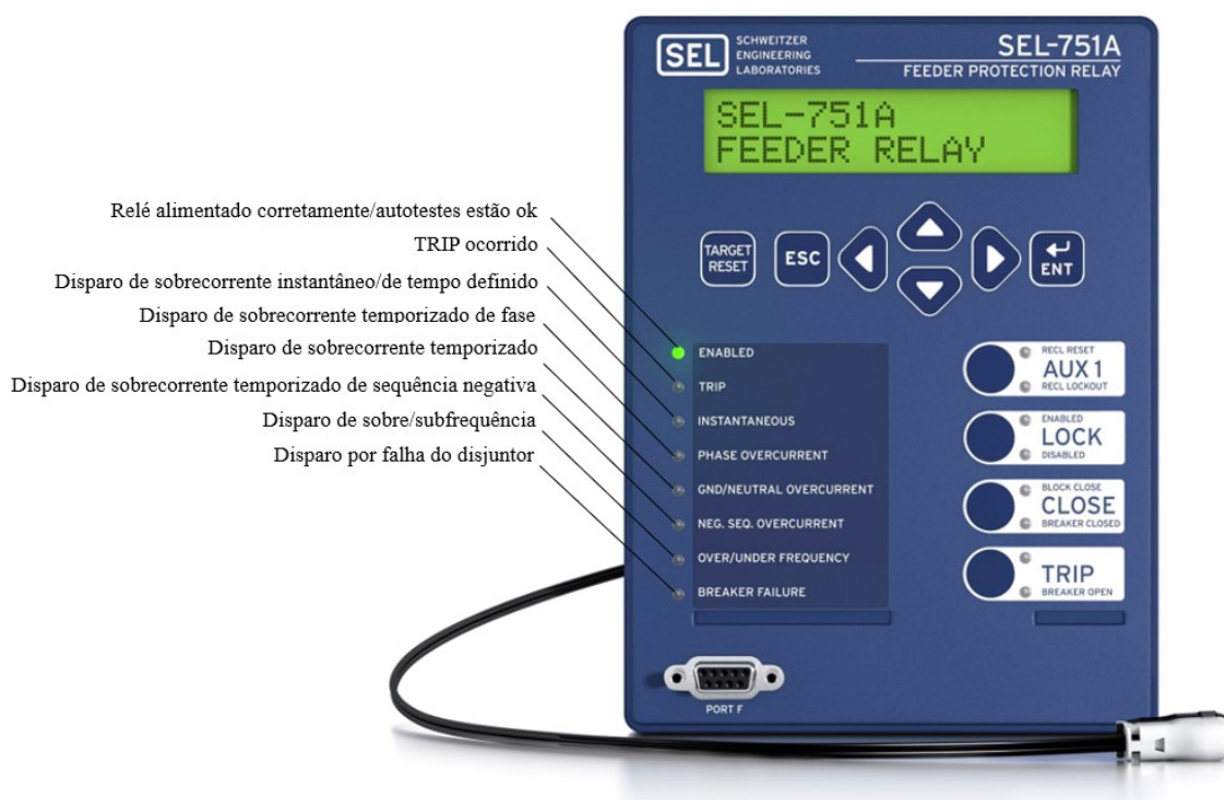
Figura 1: Layout frontal relé SEL-751A.
