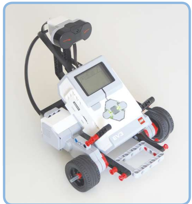
Figure 2-1: The EXPLOR3R moves around on two front wheels and a support wheel in the back.
